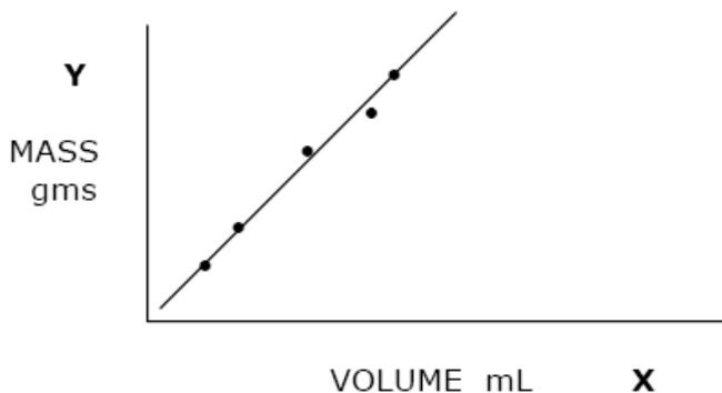
You must use data points FROM YOUR BEST FIT LINE, which do not necessarily come from your actual data tables. We will NOT use the density equals mass over volume formula for any reason during this lab. The calculations of slope will be our “average density” for all five of our measurements.
